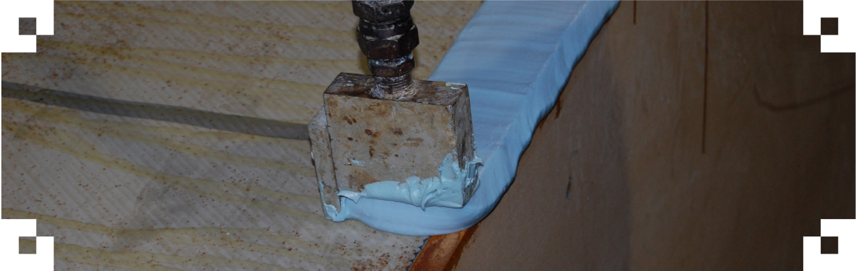
This photo shows tooling putty applied to foam surface
