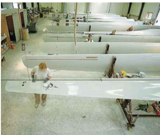
On the left Two halves of rotor blade bonded together with bonding paste.
