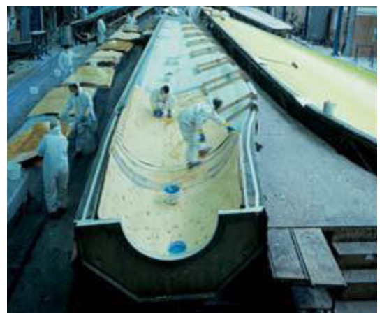
On the left Two halves of rotor blade bonded together with bonding paste.
