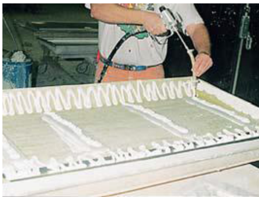
On the left Surface filler for levelling uneven surface.
