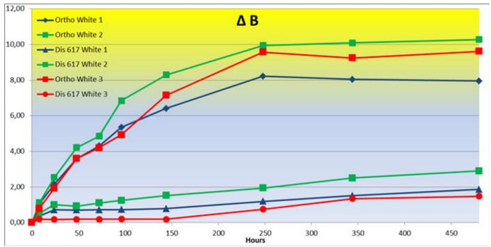
Samples were exposed to QUV-B at 313 nm cycle 4 hours at 60°C UV + 4 hours at 50°C condensation according to ASTM G 154 Cvcle 2 : exposure up to 480 hours
